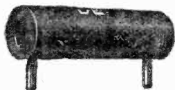
Fixed resistors are both neat and easily changed.
